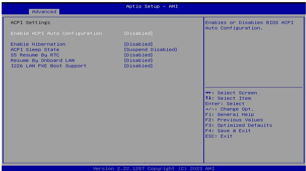
[Resume By onboard LAN] This option is used to set up Wake-up on LAN.
