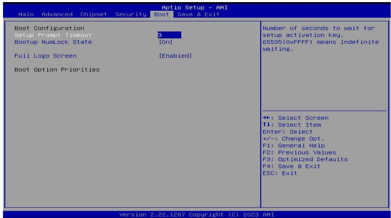
[Setup Prompt Timeout] This option is used to set the length of time the POST interface stays on.
